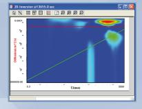
Nuclear Magnetic Resonance (NMR) logging is now established as part of the modern logging suite. Nevertheless, while logging hardware has made major advancements, software for interpreting NMR data is not widely available. LogIC is one of the few software packages available in the industry with full NMR log interpretation capability, and perhaps the only software having the ability to incorporate both NMR core analysis data and geological reasoning into the interpretation.
